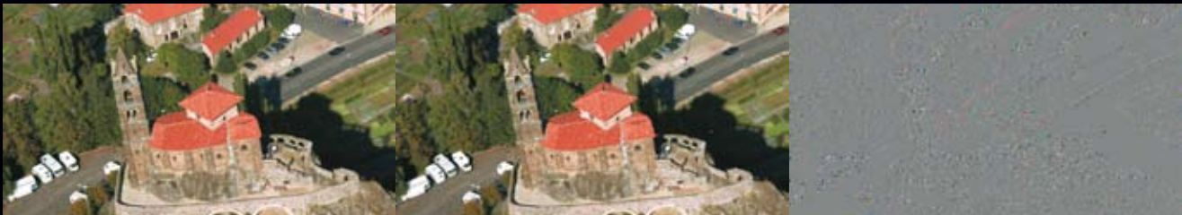
Left: Original image Center: Intra-frame predictive image Right: Difference image obtained from subtracting the intra-frame predictive image from the original image. This shows the high accuracy of intra prediction.
